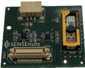
**GAP Sensor Module:** It provides the complete solution for motion and positioning applications. It houses a GPS transceiver with an integrated antenna, an accelerometer and an interface for a PIR sensor
