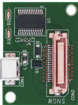
**USB Gateway Module :** It programs the microcontroller and acts as an interface between the network and PC.
