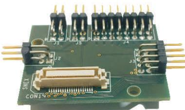
**Extender Module:** It extends all the pins of the micro controller on a board and provides access to users, if needed. This makes it easier to,
