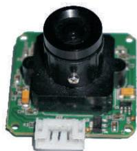
**Camera Module:** it supports QVGA/160\*120 resolution output in JPEG
